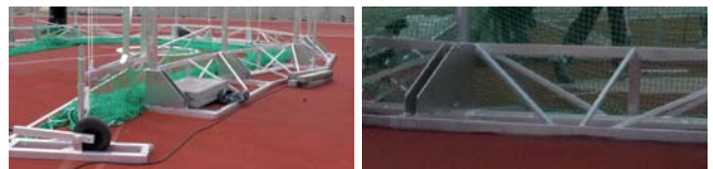
Makes the cage mobile: the socket frame.
